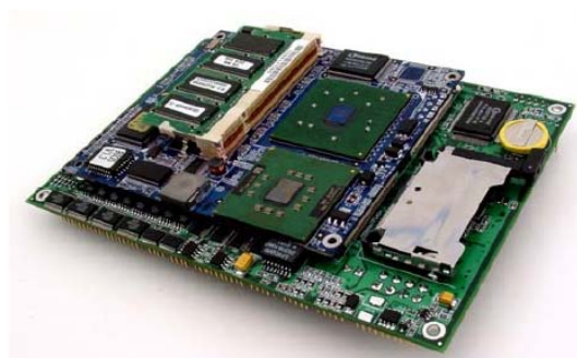
PLT-BASE: ETX form-factor development baseboard for the ETX-945 Series
