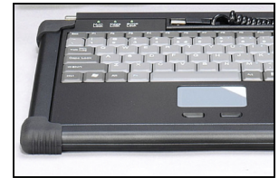
Keyboard with integrated 2-button touchpad
