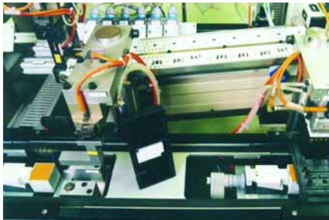
Use of MOBY devices on an assembly line producing SIRIUS contactors at Siemens Amberg
